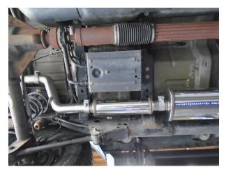
**Step 3.** Install the Resonator to the Muffler Assembly using the supplied clamp.
